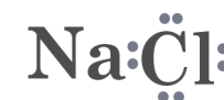
Figure 19.9: Sodium and chlorine form an ionic bond. The compound sodium chloride is electrically neutral as long as the two ions stay together.
