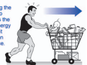
Figure 5.7: Kinetic energy depends on two things: mass and speed. The amount of kinetic energy the cart has is equal to the amount of work you do to get the cart moving.
