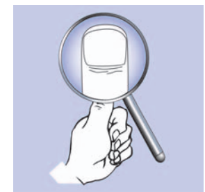
Figure 15.6: A magnifying glass makes a virtual image that appears larger than the object.
